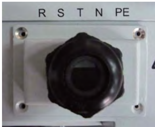
Fig.11 - Terminal board for AC cables connections
